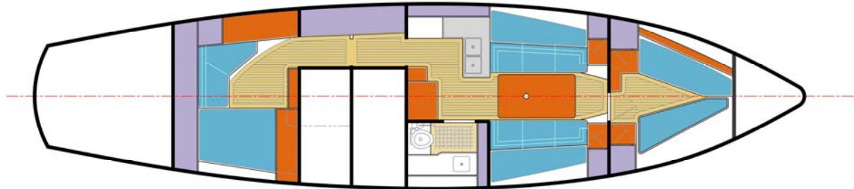
Design Number 0604 Via Maris a large walk-in engine room beneath the doghouse
