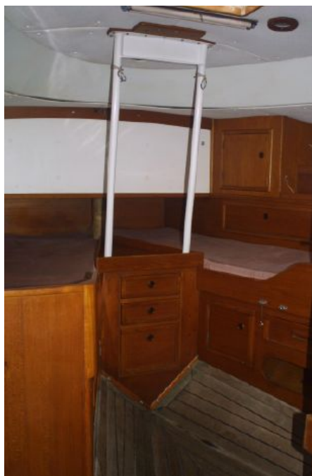
The aft cabin Moody 44 , standard layout of the production yacht. Twin pillars support the mizzen mast
