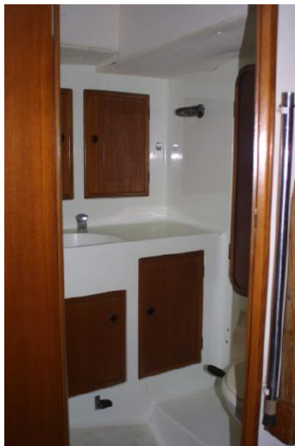
Aft head Moody 44 , the head compartments are built on Separate internal F.R.P mouldings.
